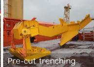
Trencher makes multiple passes within the existing trench No part of trencher near the cable provides low risk solution for the cable
