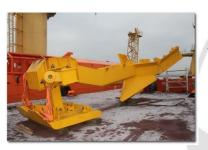
SCAR 1 - Pre-cut trenching (multi-pass) - Route preparation / boulder clearance
