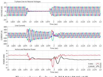
Three phase fault on 2.75MW PMG WT (source: http://www.nrel.gov/docs/fy15osti/62998.pdf)
