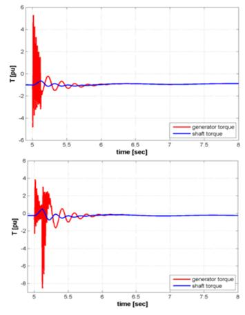
Powertrain torque during single phase (top) and three phase (bottom) grid fault
