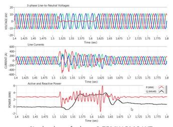
Single phase fault on 2.75MW PMG WT (source: http://www.nrel.gov/docs/fy15osti/62998.pdf)
